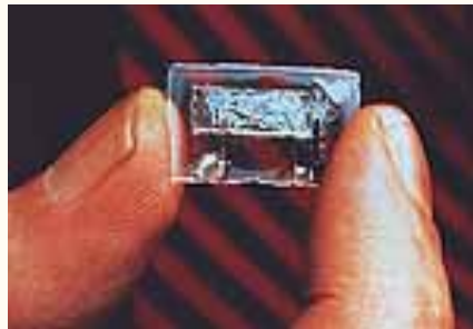
Kilby' s first integrated circuit
